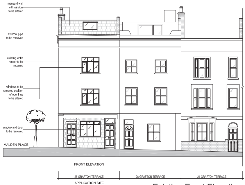
Existing Front Elevation
