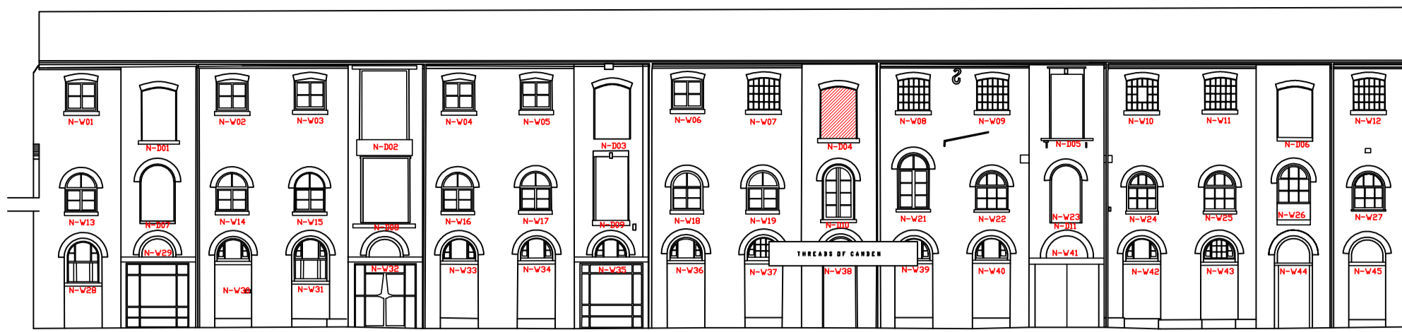
Existing north elevation Scale 1:200 Type 1 openings identified above by red hatching.
