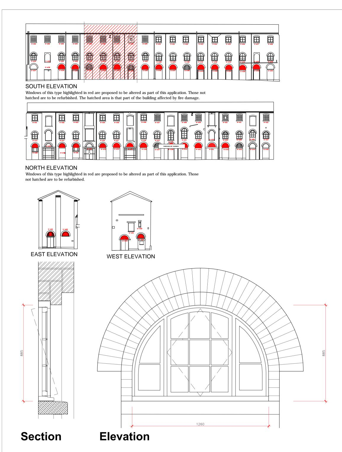
Existing fixed light / opening casement timber window - Scale 1:10
