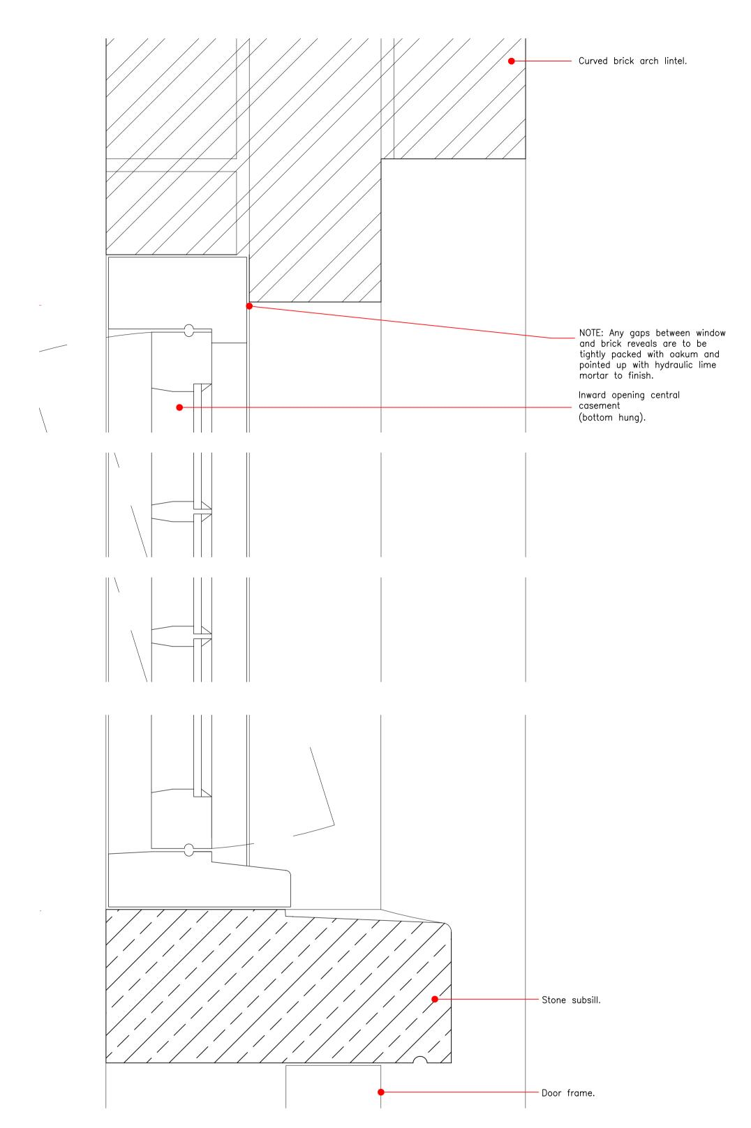
Existing fixed light / opening casement timber window - section Scale 1:2
