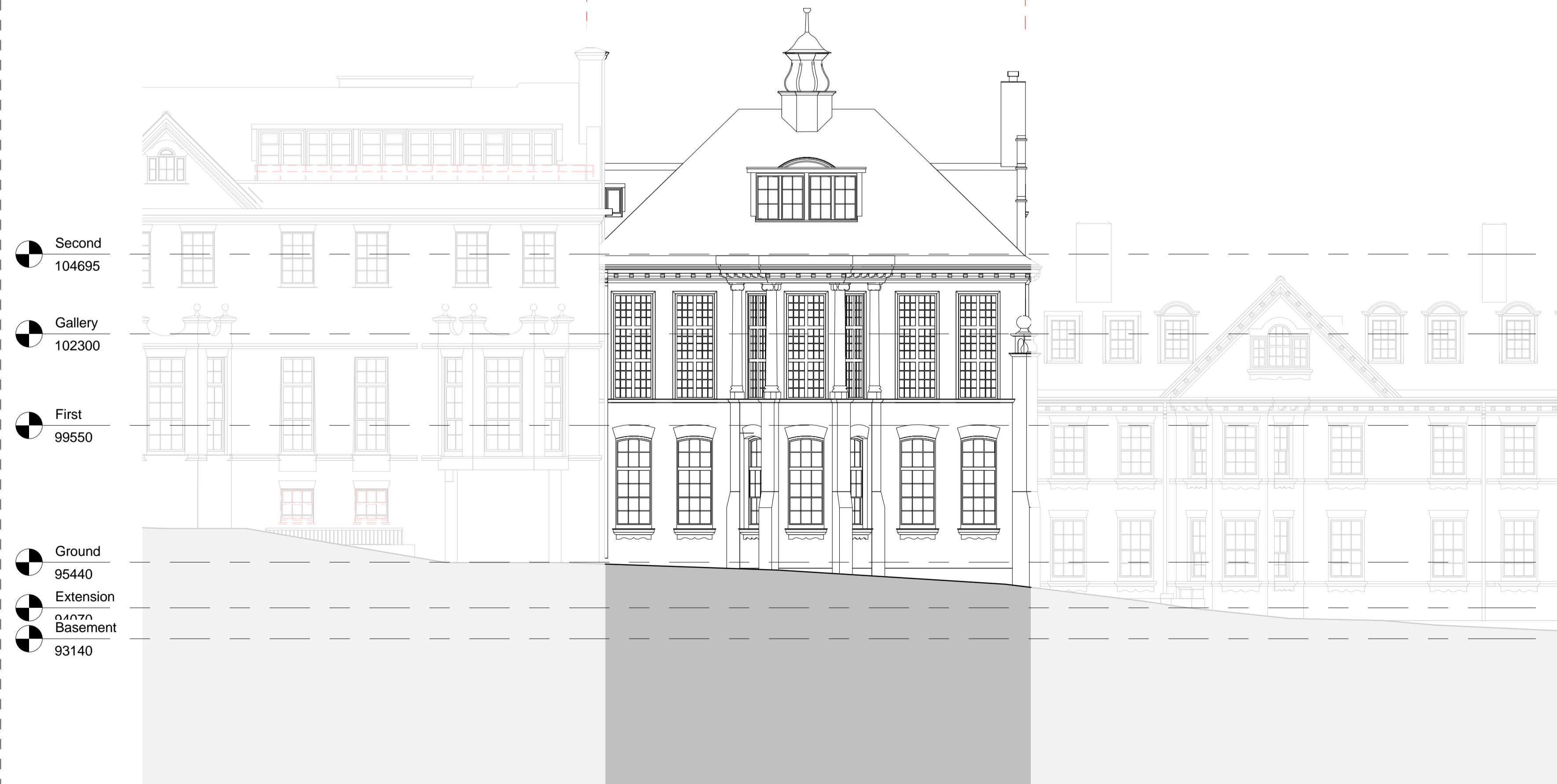
2 Proposed South-West Elevation 1 : 100
