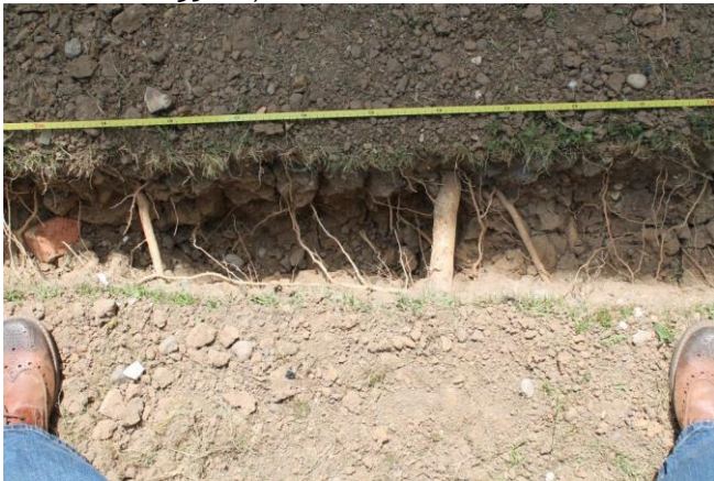
Photo 3. Between 1m and 2m from the monitoring point were roots of 35mm, 20mm and 20 roots of 2mm to 8mm
