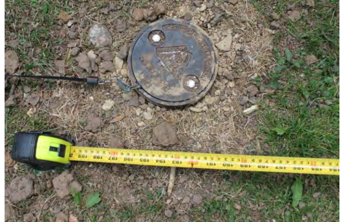
Photo 2. Monitoring point at 0.9m from the end of QMH dictated the max extent of the trenching. Smaller tape is to allow the roots to be plotted.
