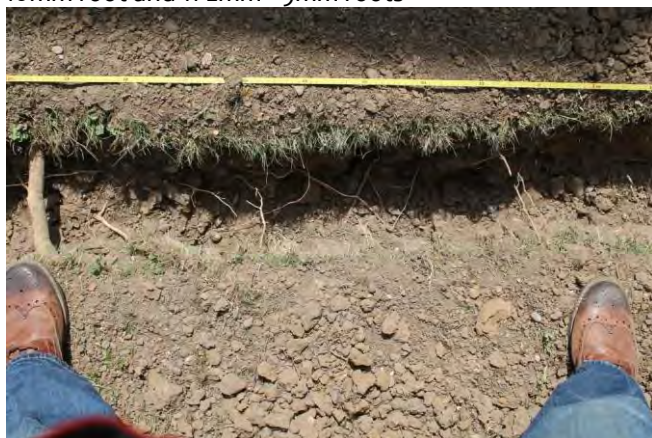
Photo 5. Between 3m and 4m were one 30mm root, one 10mm root and 11 2mm - 9mm roots
