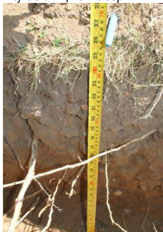
Photo 17. Maximum depth of trench is 67cm. Minimal rooting activity below 40cm deep
