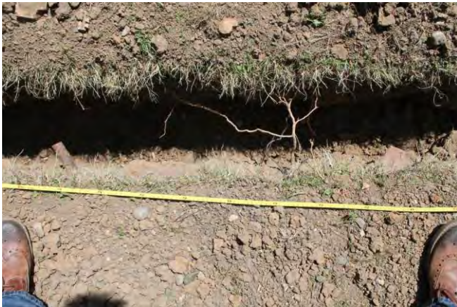
Photo 9. Between 7 and 8m from QMH only one root dia 8mm.
