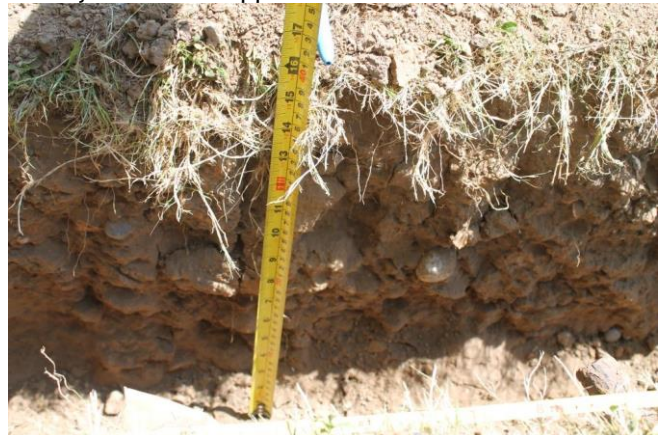
Photo 18. Shallowest part of trench is 42cm deep. this was distant from the ash where there was no rooting activity even in the upper soil bhorizons.
