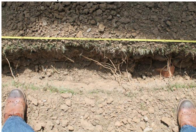
Photo 4. Between 2m and 3m were 14 roots between 2mm and 10mm plus several fibrous roots.
