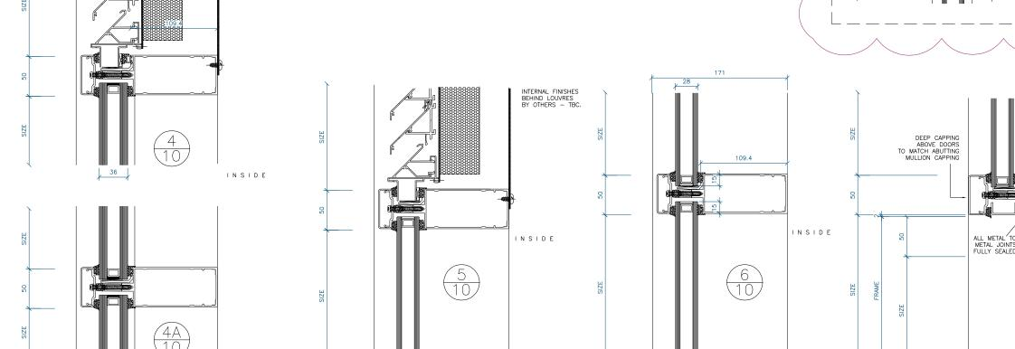
GENERAL NOTES: PERIMETER OF ELITE FRAMES TO BE EXTERNALLY SEALED TO SURROUNDING STRUCTURE.
