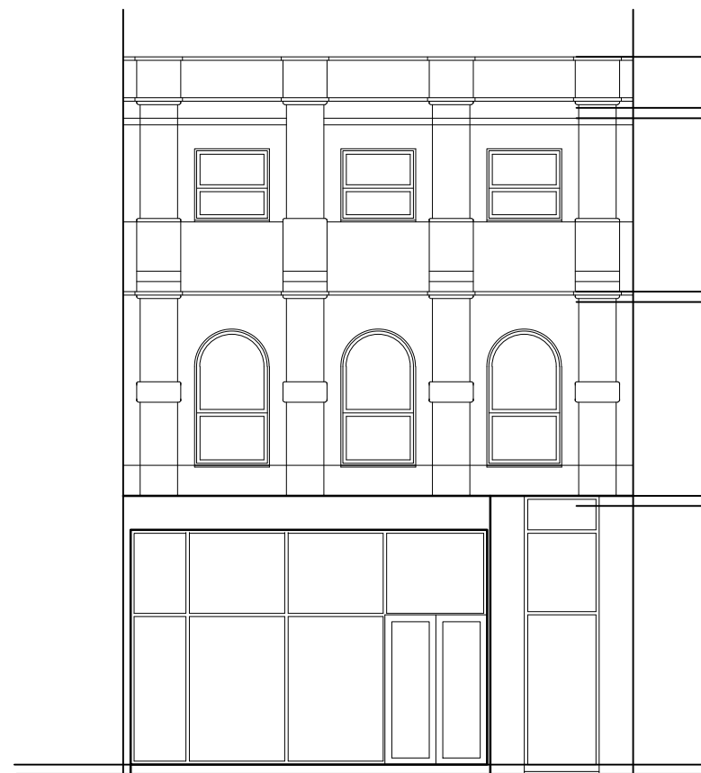
PROPOSED FRONT ELEVATION (CLADDING TO MATCH EXISTING RENDER)
