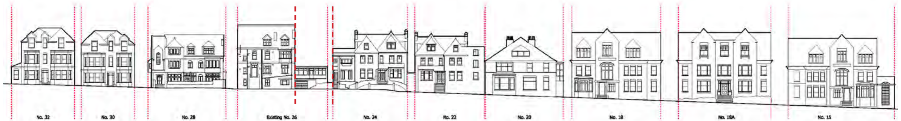
Fig. 4.5.4 Elevation showing widths between buildings, existing
