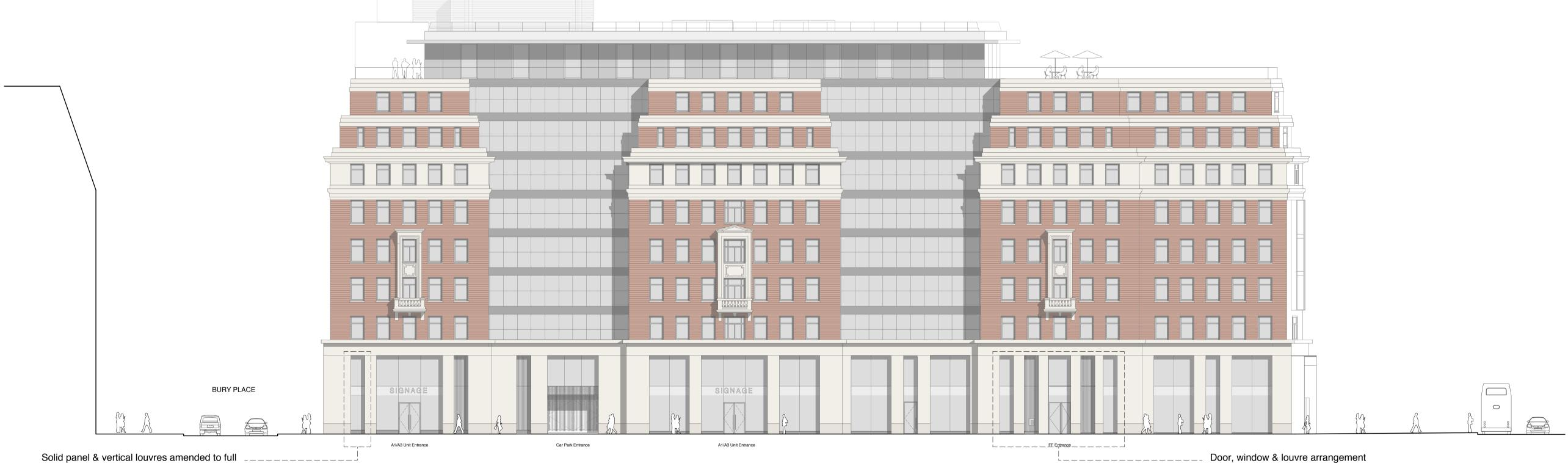
Solid panel & vertical louvres amended to full height glazing; detail to match existing
