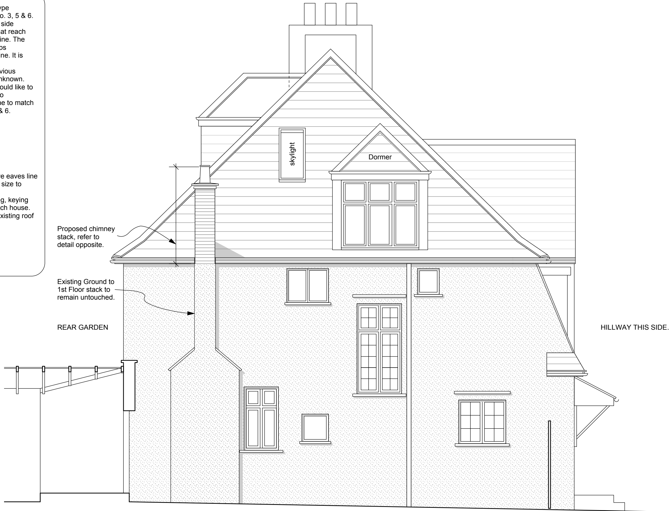
PROPOSED SIDE ELEVATION (scale 1:50 @ A3)
