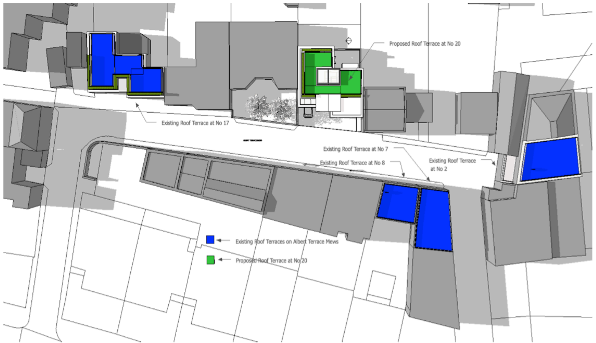
Fig.8 – 3d images showing the presence of existing roof terraces in Albert Terrace Mews in addition to the proposed roof terrace.
