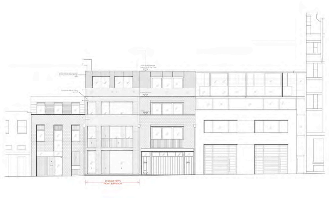
proposed façade drawn in context of consented schemes; granted for adjacent properties at numbers 25, 26, 28, 29 and 30 King's Mews
