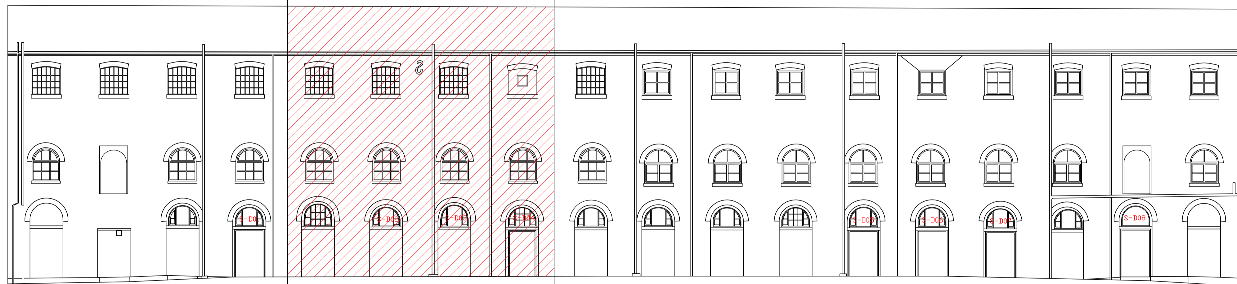
South Elevation as Existing (Hatched area denotes fire damage)
