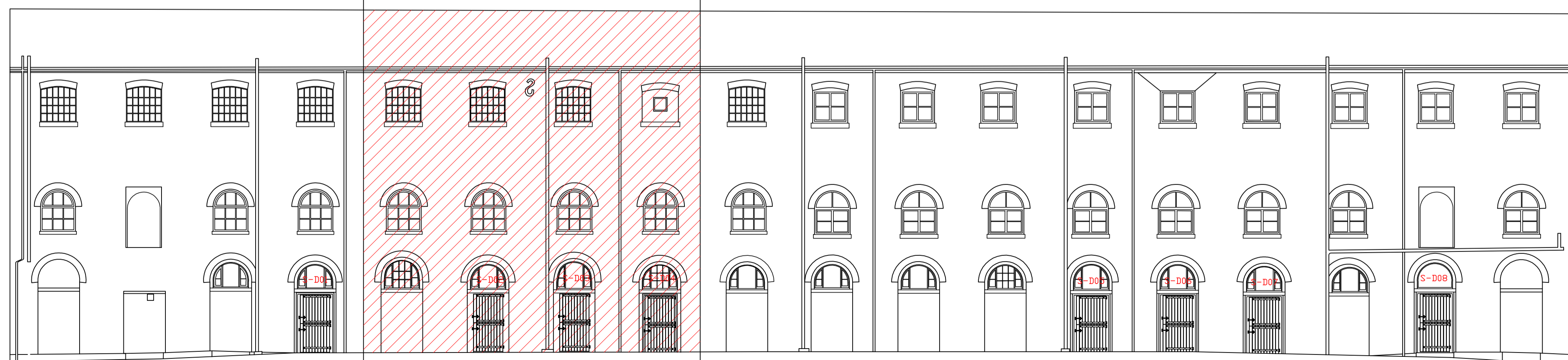
South Elevation as Proposed (Hatched area denotes fire damage)
