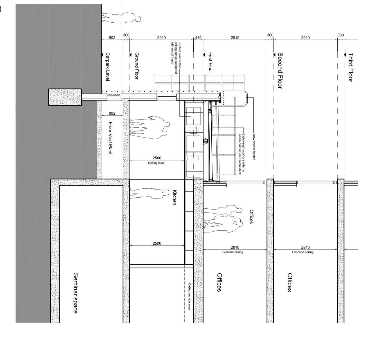
Section B: Proposed section through new kitchen extension
