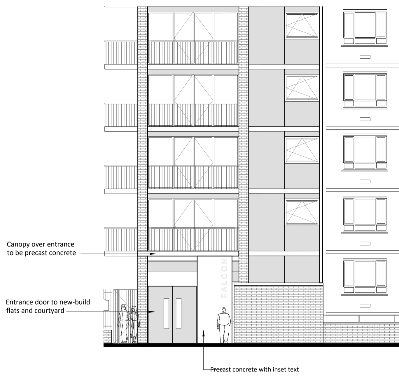
SW Detail Elevation showing Entrance 1:100
