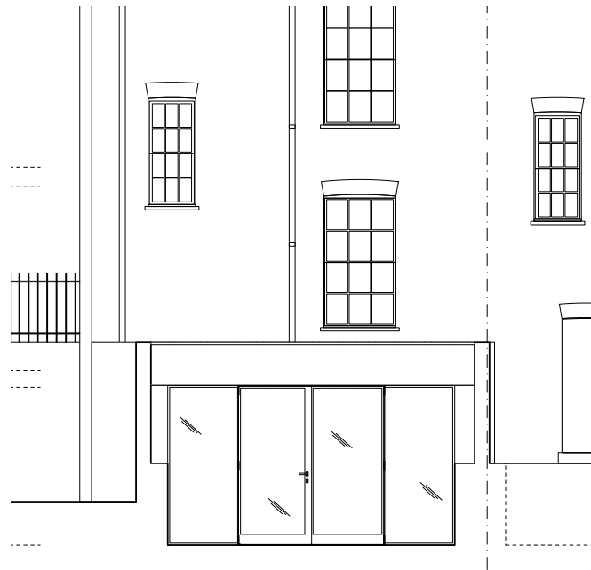
fig4. Proposed elevation of rear extension.
