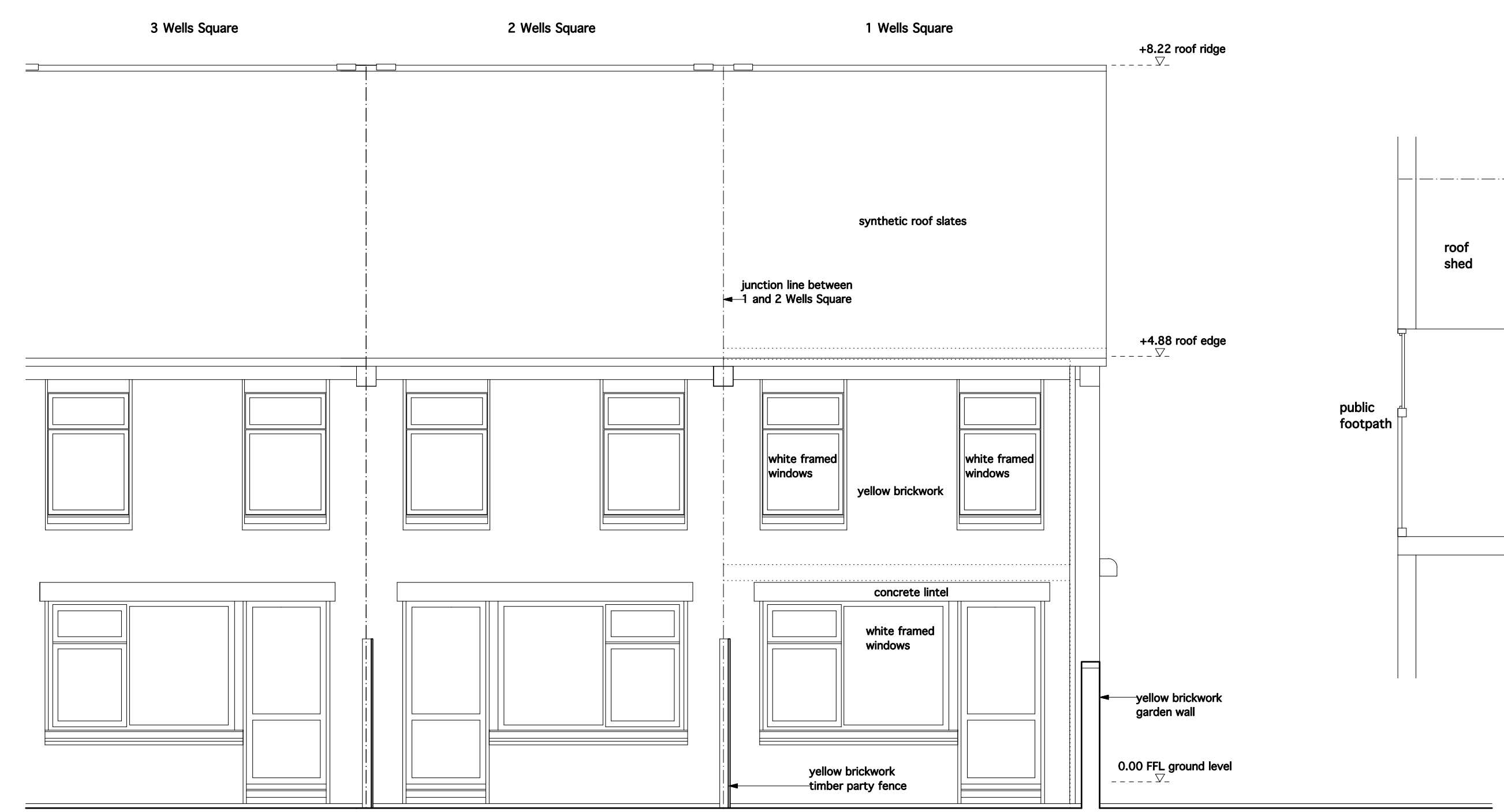
rear elevation existing in context 1:50
