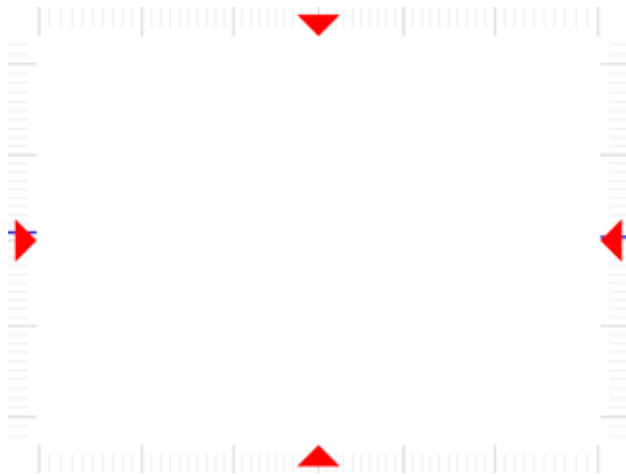
Sample graticule showing optical axis markers
