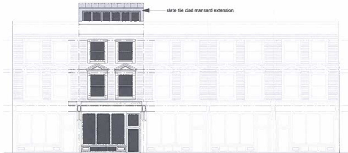
front elevation as existing
