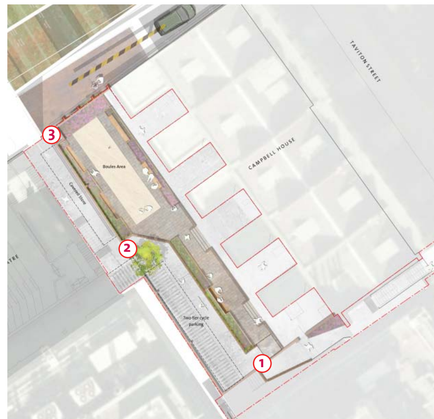
(2) 4.4m long section to be removed in western wall
