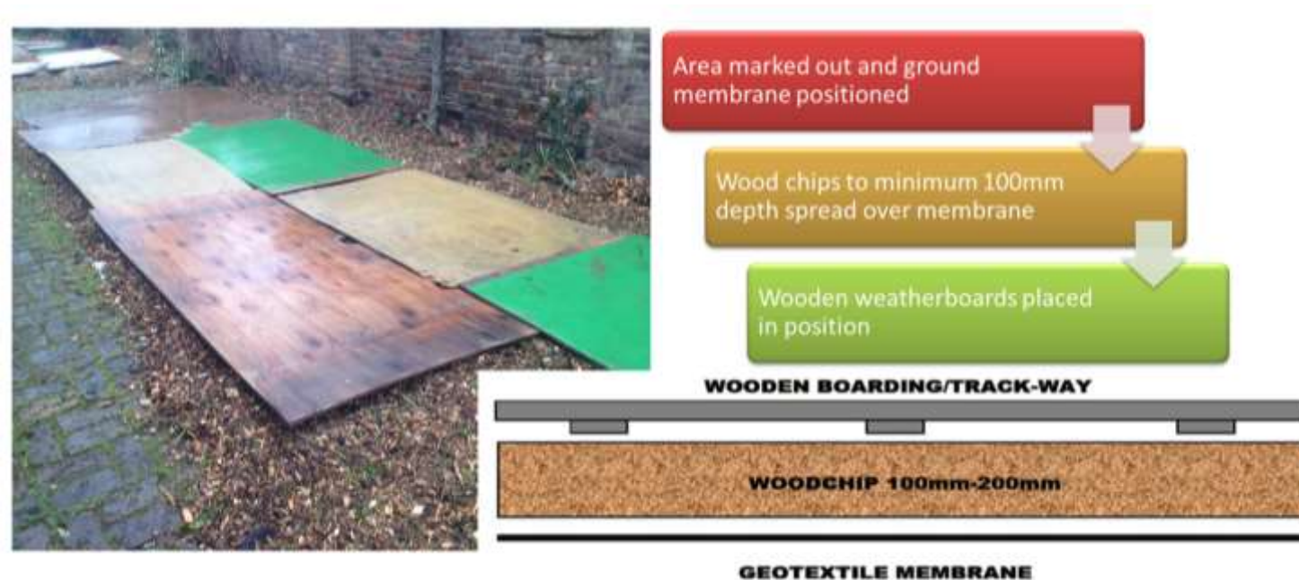
Fig 2 - Temporary ground protection detail
