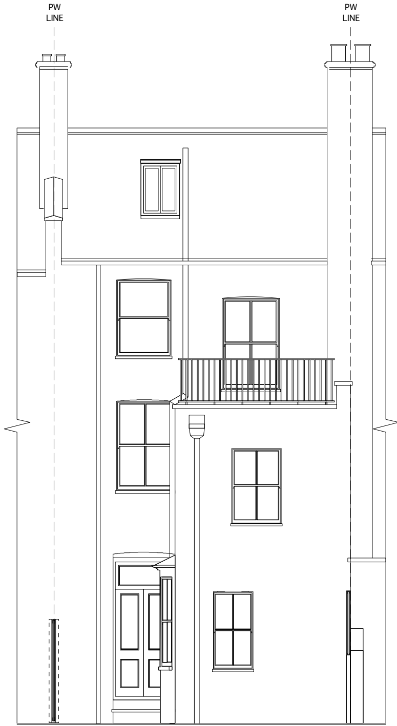
REAR ELEVATION AS EXISTING
