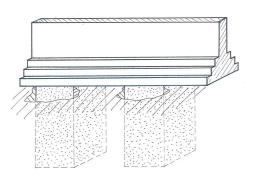
Stage 2c: excavation and concreting of an intermediate section, to form contiguous rows of underpin
