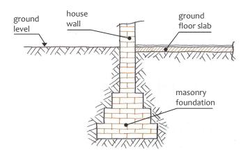
Stage 1: exposure of original foundation by digging a short trench along a section of the wall to be underpinned
