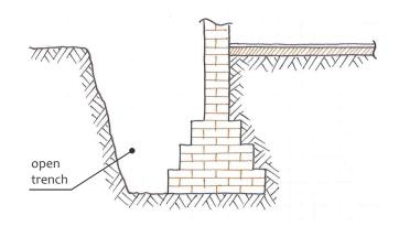
Stage 2: excavation of pit to form underpin: see Fig. 2.1b for details
