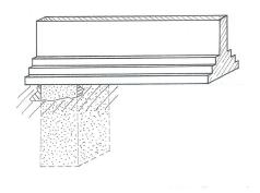
Stage 2b: excavation and concreting of another section, not adjacent to first one
