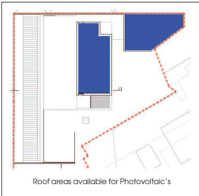
7.2.2 As the diagram shows, a number of roof sections were identified as suitable for installation of photovoltaic panels. From this review it was identified that a maximum area of 197m<sup>2</sup> is available for any proposed photovoltaic installation.
