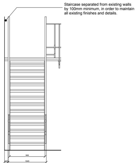
FIRST FLOOR STAIR: ELEVATION 1
