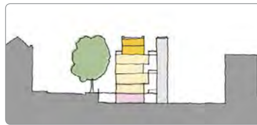
Section demonstrating Troutbeck overbuild capacity
