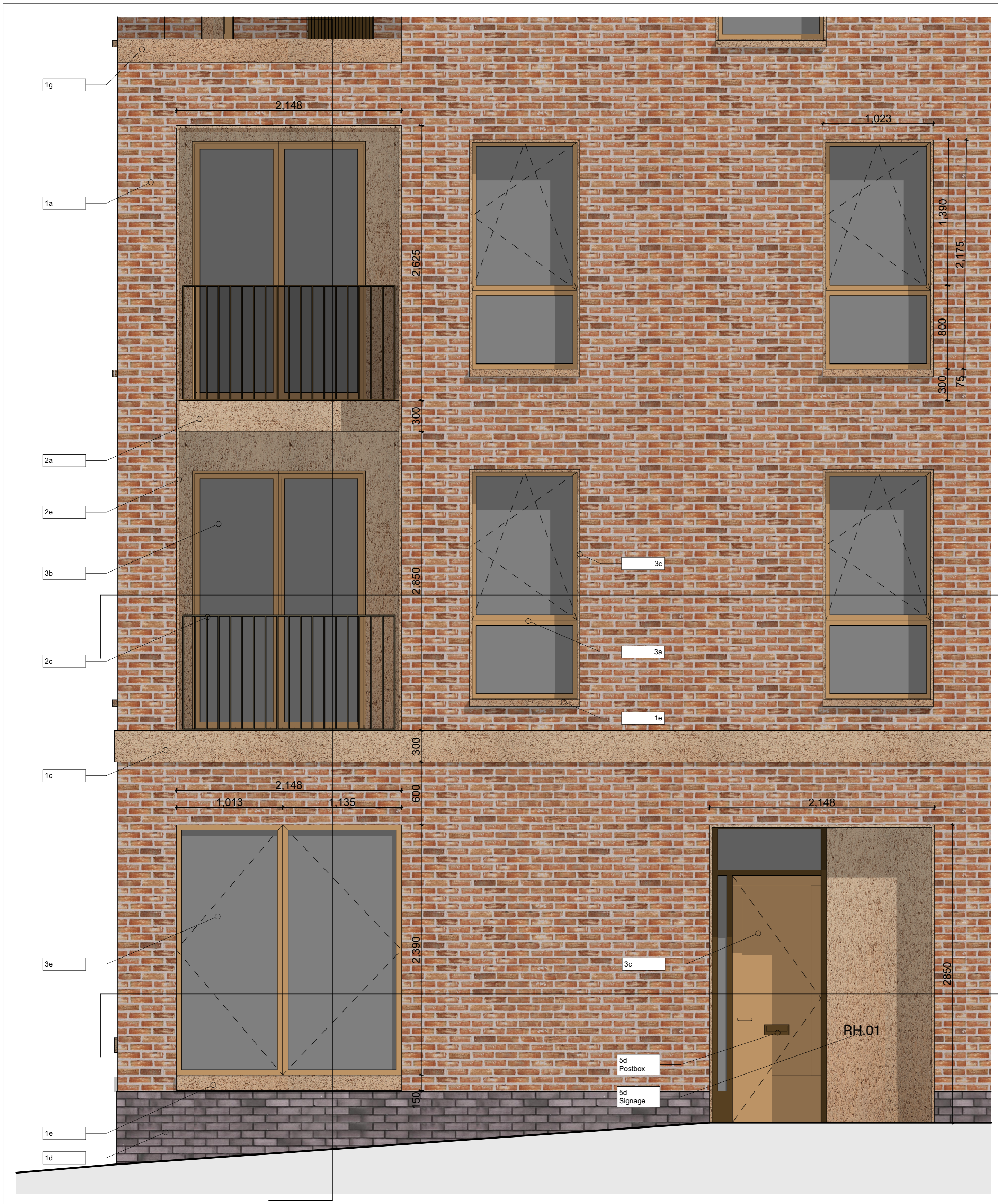
S5-402_01 Typical Bay Elevation 1:25
