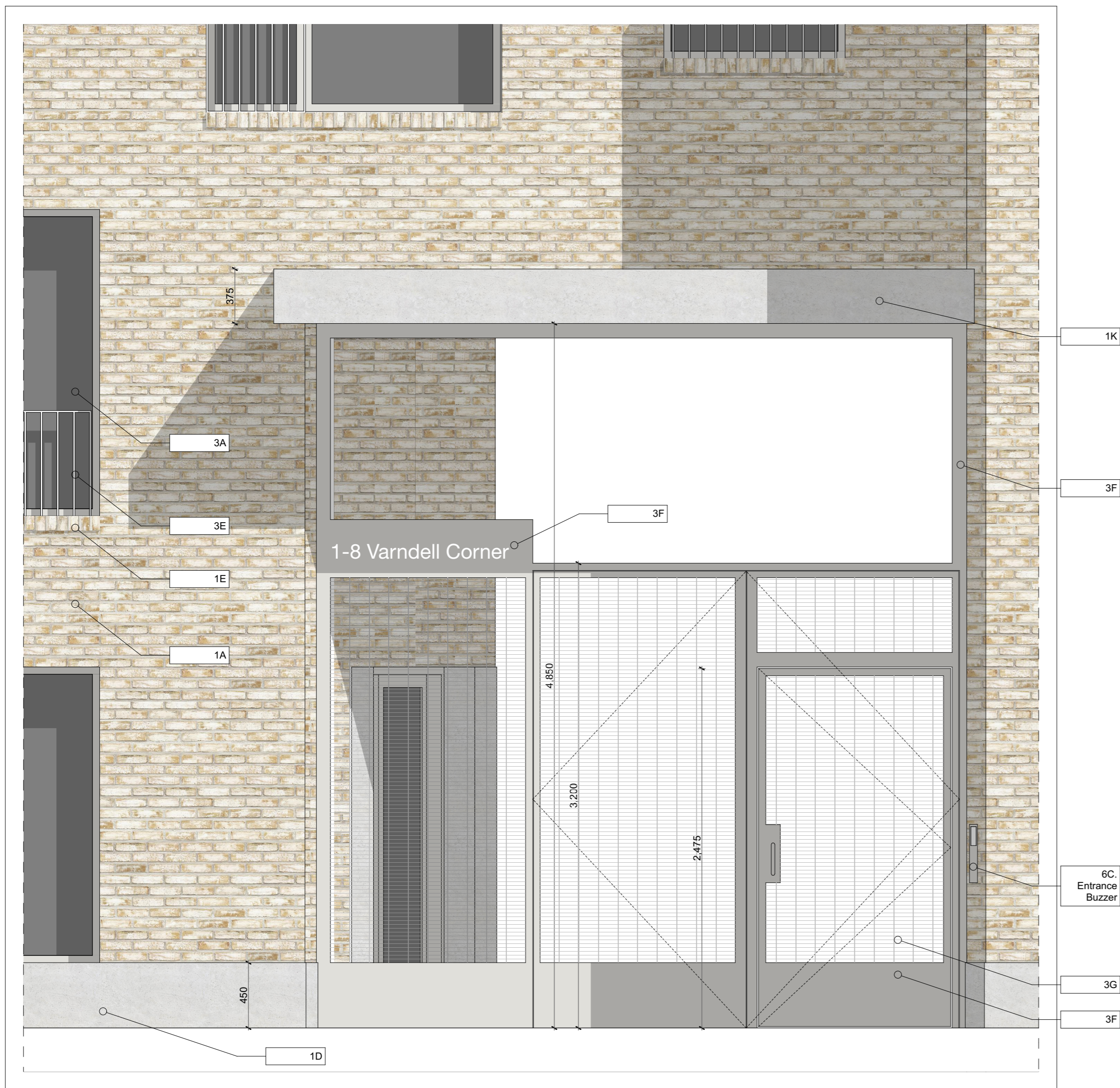
A-S3-402-01 Communal Entrance Gate Elevation 1:25
