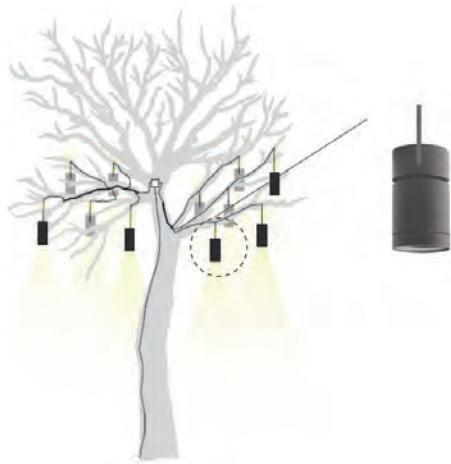
Lighting to existing mature trees
