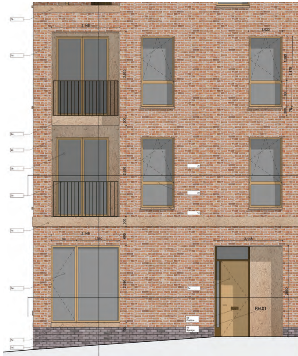
A - Typical Bay, with Domestic Entrance and Recessed Balconies
