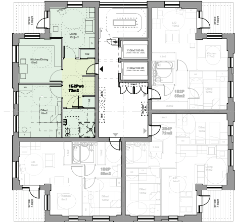
Floor Type C - upper duplexes with a possible 1Bed wheelchair unit option
