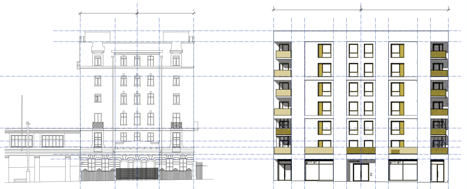
Study of proportions and hierarchy, drawing on the National Temperance Hospital, to create a modern mansion block opposite at the One Stop Shop site.
