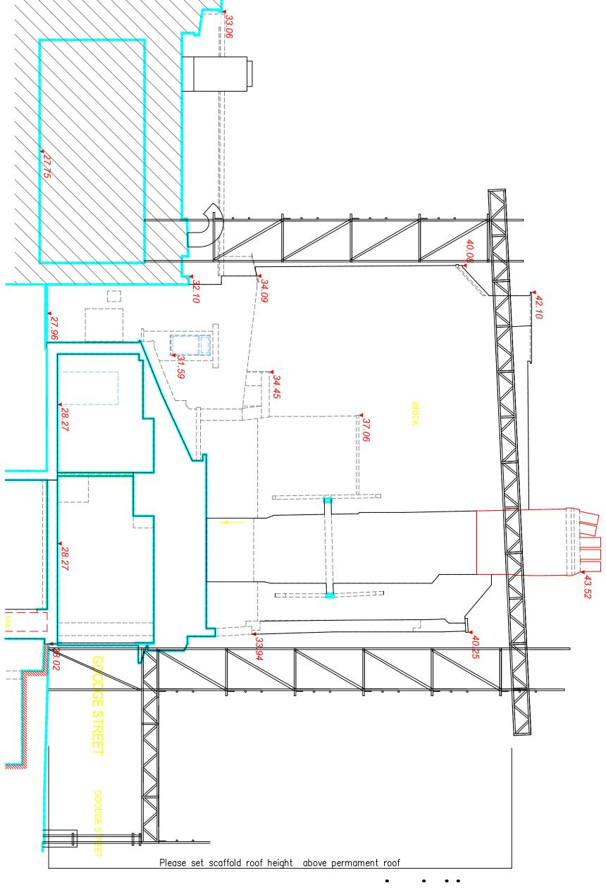
Scaffold based on typical 2m high lift Gantry level to be at shop signs level 3.450m above street level Standards to located on the sides of access door (required access to Site,Subway,STA Travel)
