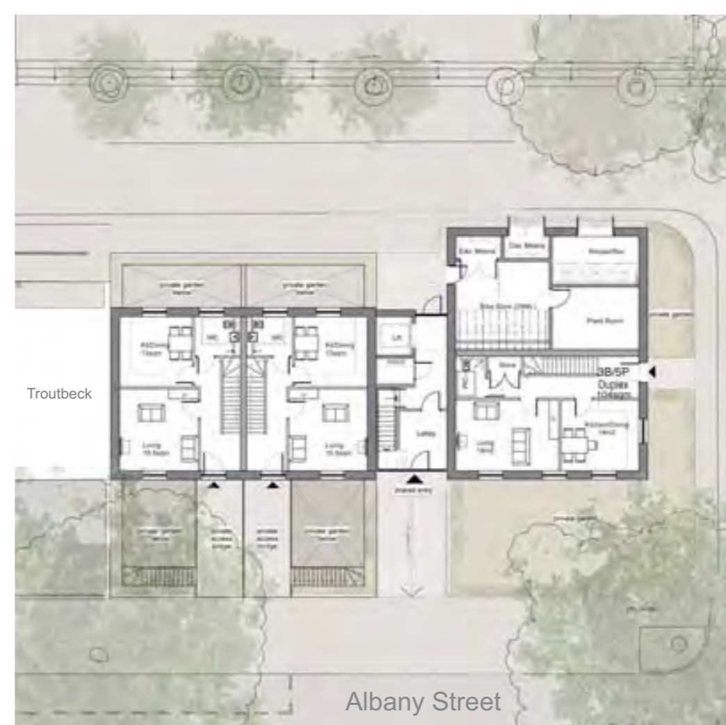
Ground Floor plan, showing duplexes entering off the street, and the main residential entrance on Albany Street
