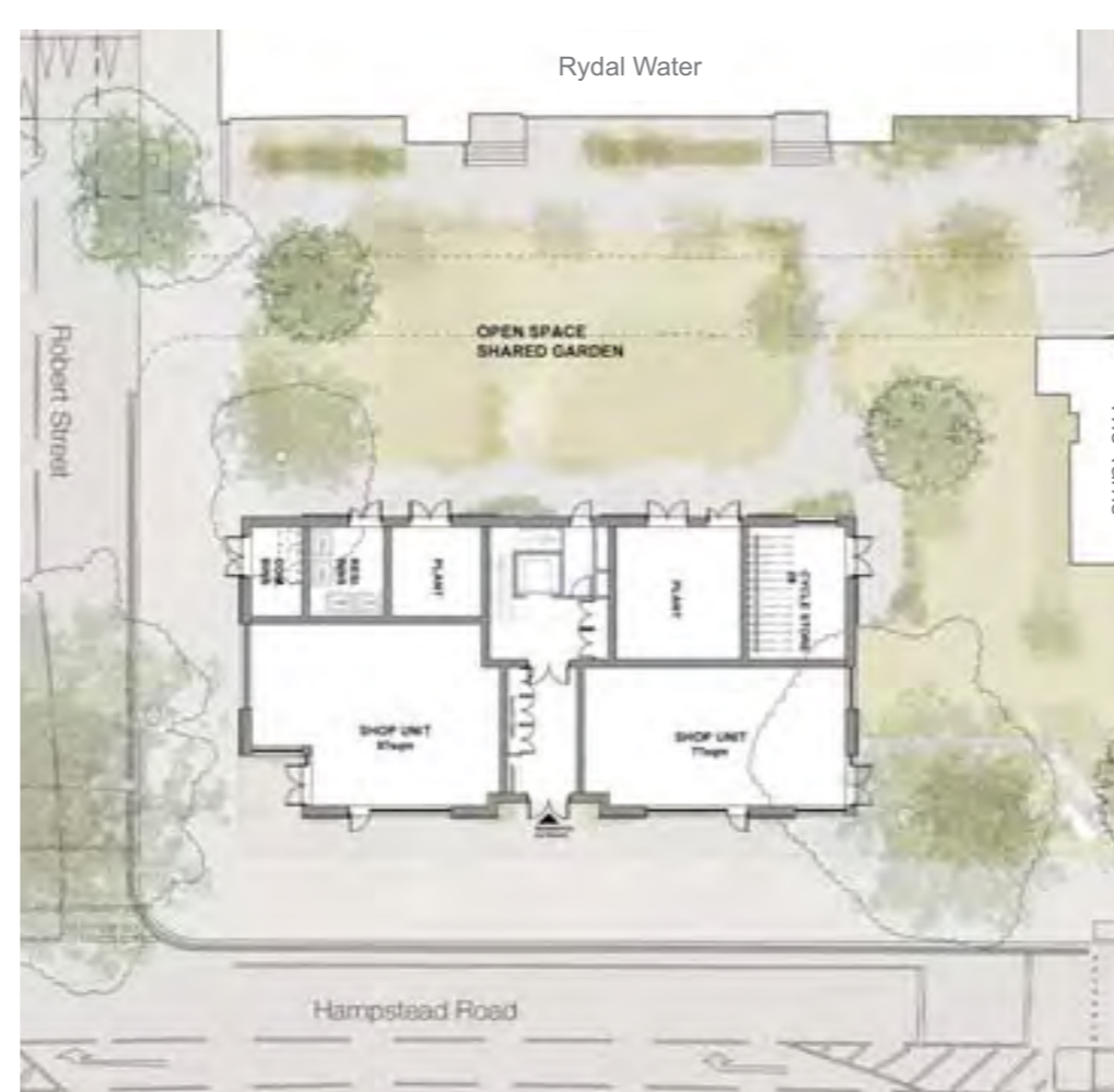
Ground floor plan, showing the main entrance to the flats on Hampstead Road, with two shop units either side
