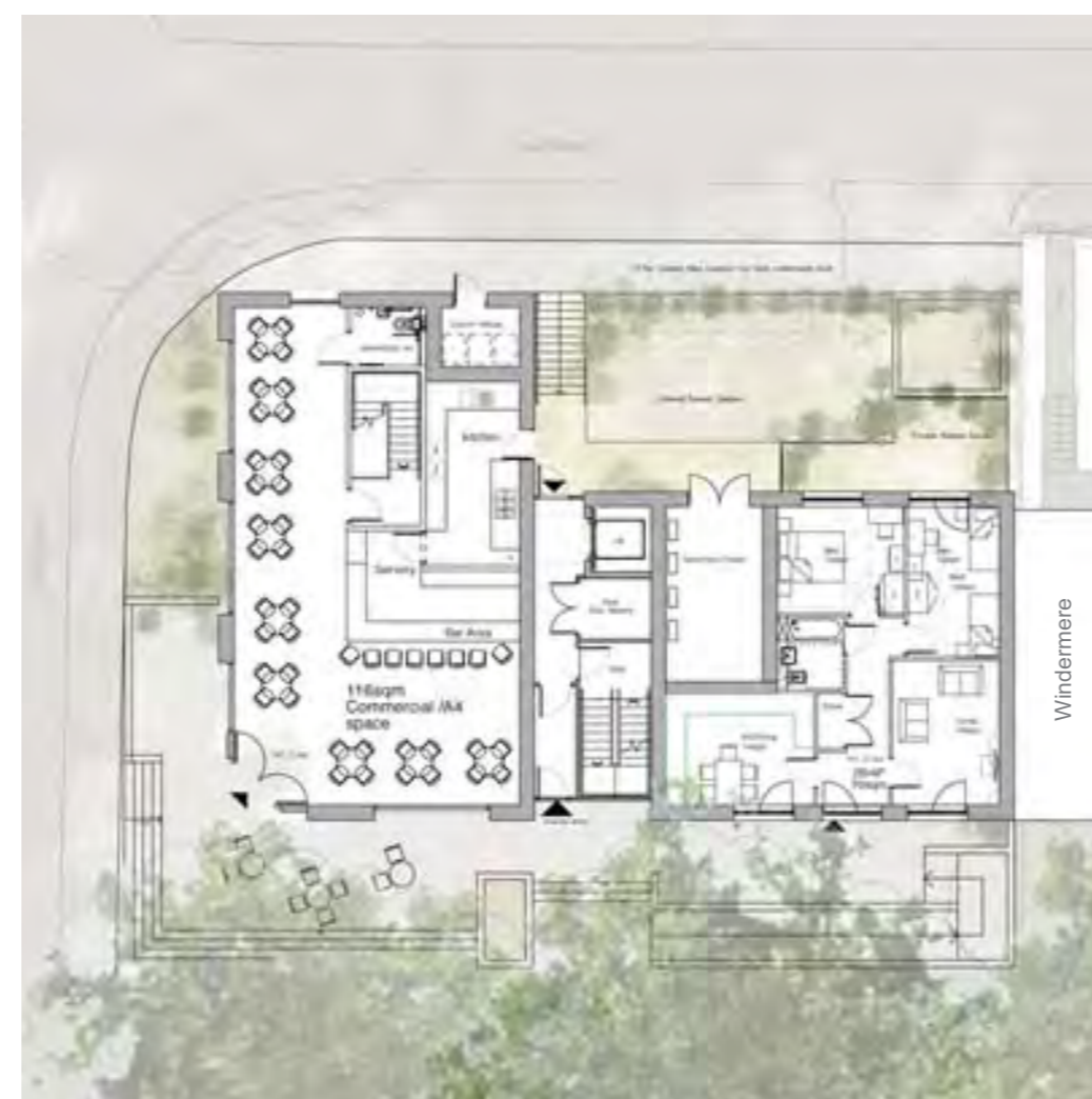
Ground Floor Plan, showing a pub on Nash St corner, a 2-bed flat with a private terrace, and a shared garden on the east side
