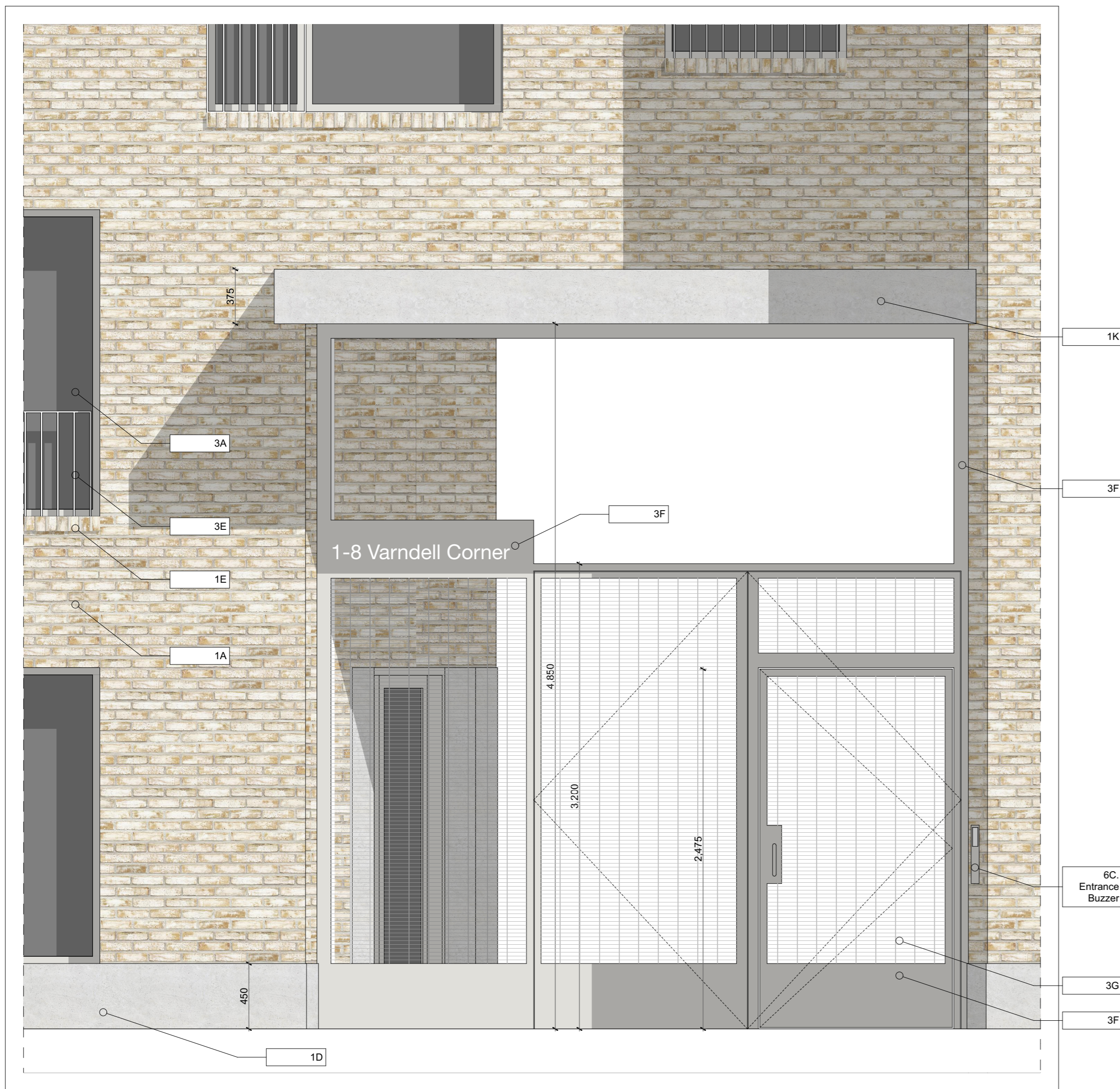
A-S3-402-01 Communal Entrance Gate Elevation 1:25
