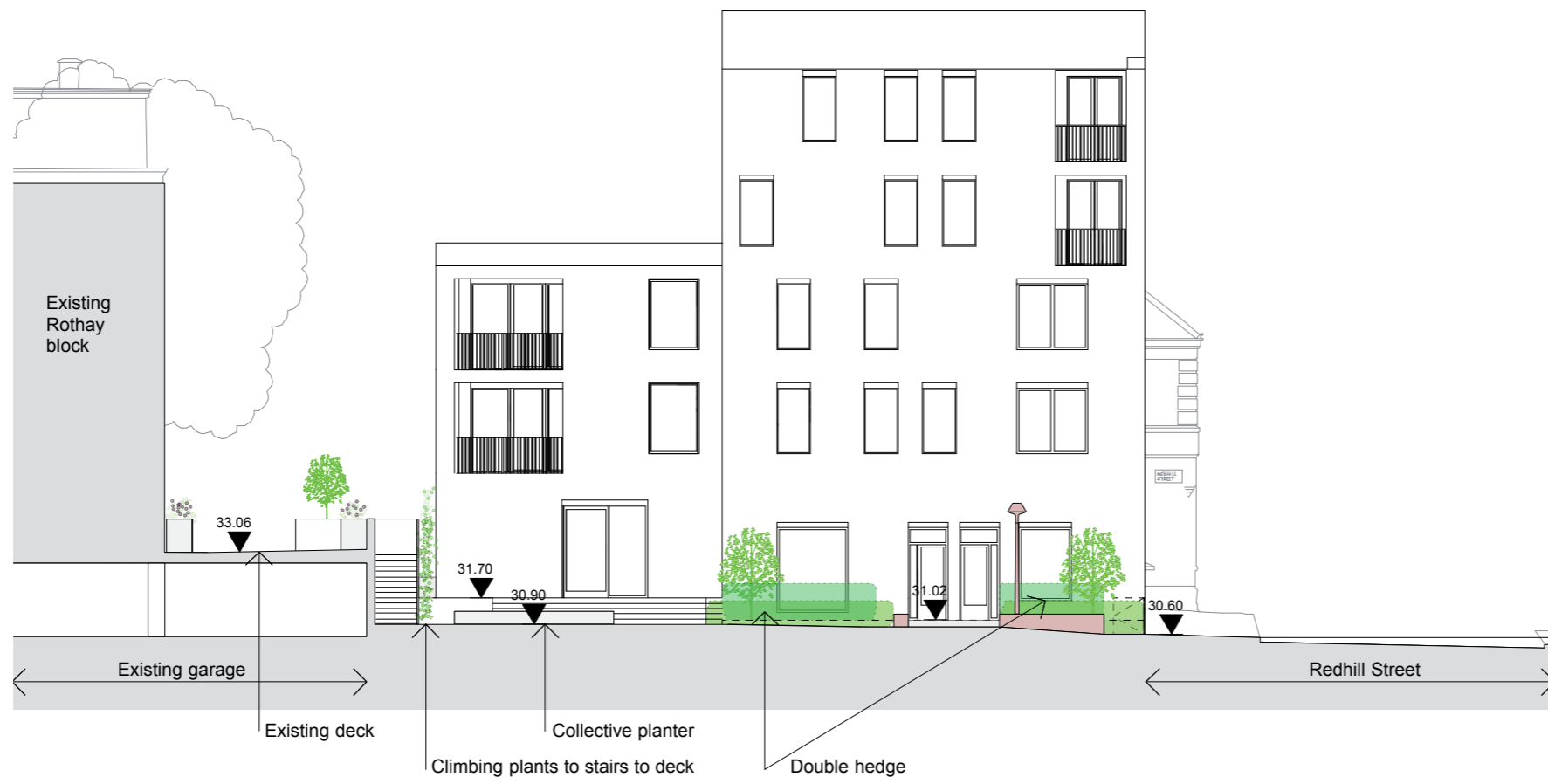
Cross section AA along north facade
