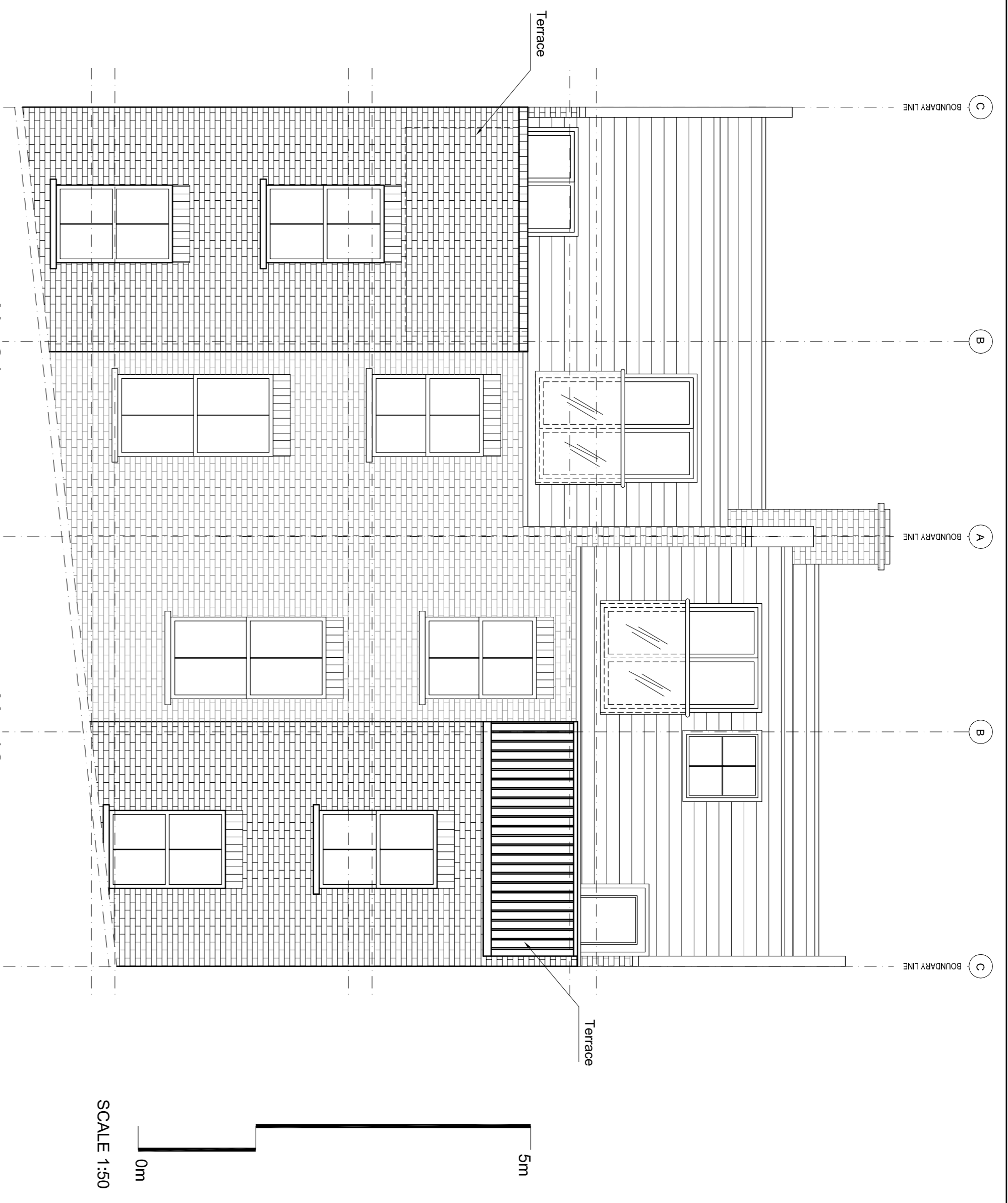
02: PROPOSED REAR ELEVATION No 19-21 SCALE 1:50
