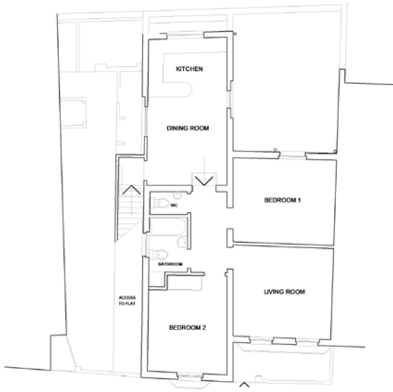
EXISTING FIRST FLOOR PLAN Gross Area = 88.15 sqm
