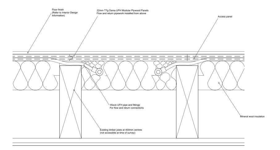
NOTE: Plywood subfloor panels to be laid staggered
