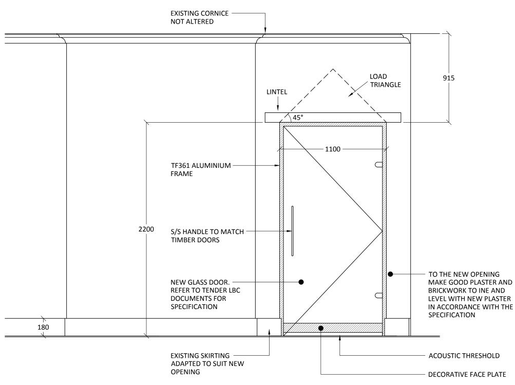
MASONARY ARCHING ACTION MEANS THAT ONLY THE MASONARY WITHIN THE LOAD TRIANGLE (INDICATED ABOVE) IS CARRIED BY THE LINTEL. LOAD FROM THE MASONARY OUTSIDE OF THIS TRIANGLE IS CARRIED BY THE WALL EITHER SIDE OF THE OPENING
