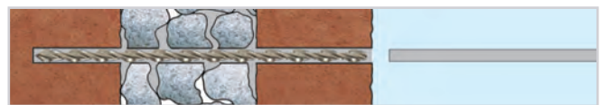
4. Back pressure pushes nozzle out of hole to leave fully grouted tie
