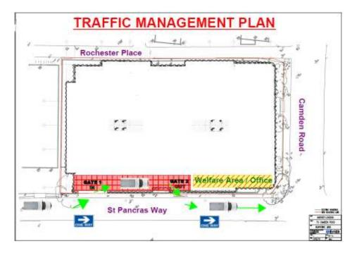
Phase 2: This stage sees the development of the New Welfare take place in Rochester Place. Pedestrian Access shall remain throughout as the Hoarding is erected. Meanwhile no changes are made to the current arrangements in St Pancras Way. This will be between 1<sup>st</sup> and 20<sup>th</sup> May 2015.
