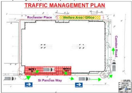
Phase 4:- At this stage from early September 2015, there is no longer any access onto the site for Deliveries as the basement has now been excavated baring access for vehicles.
