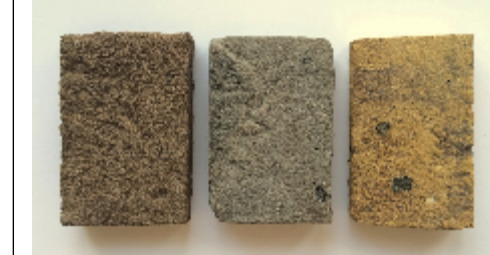
New facing brick in complementary tones and texture utilised with localised areas of re-used London stock brick.
