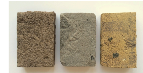
New facing brick in complementary tone and texture utilised with localised areas of re-used London stock brick.
