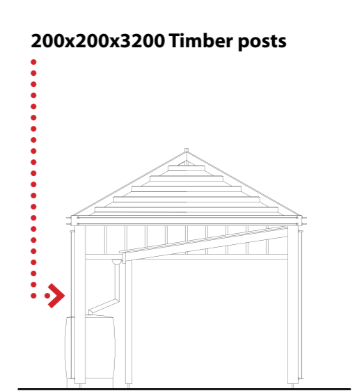
Pergola Pavilion /verandah north-south elevation 1.100
