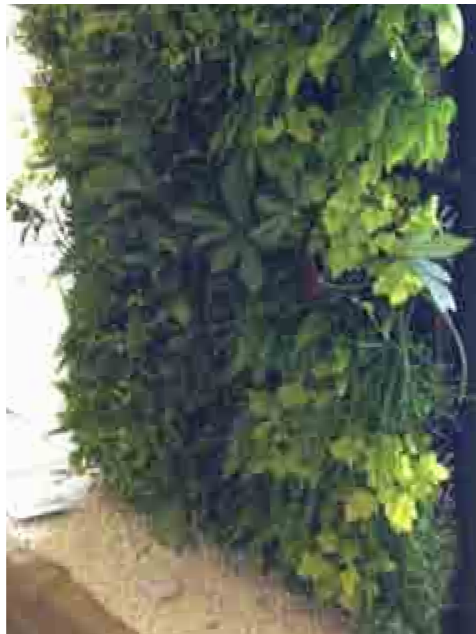
Treebox greenwall system used as vertical rain garden at rear to intercept roof water
