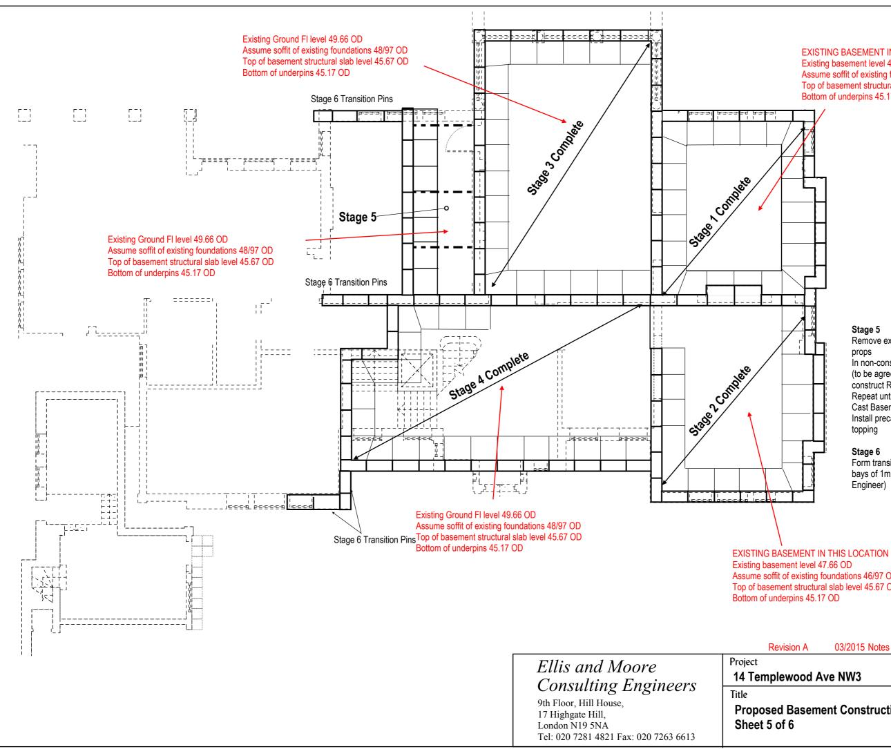
EXISTING BASEMENT IN THIS LOCATION Existing basement level 47.66 OD Assume soffit of existing foundations 46/97 OD Top of basement structural slab level 45.67 OD Bottom of underpins 45.17 OD
